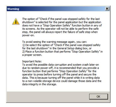
7. The software will display the following warning message when compiling a panel application if the application will save data to battery backed RAM but the software found no "Stop Operation Safely" function button in any of the application's screens. If you do not want to see the message again for the current application, click the No button in the message box. Note that the message will only display for the applications that were created with V2.0.4.11 or later.
