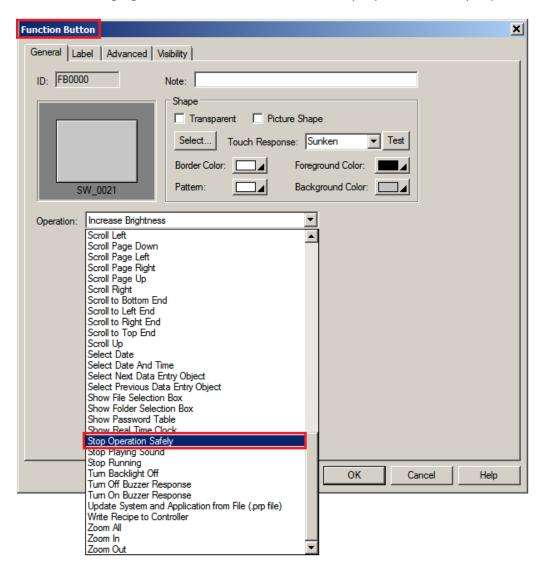
2. The HMI unit will display the following message when you press a "Stop Operation Safely" function button.
